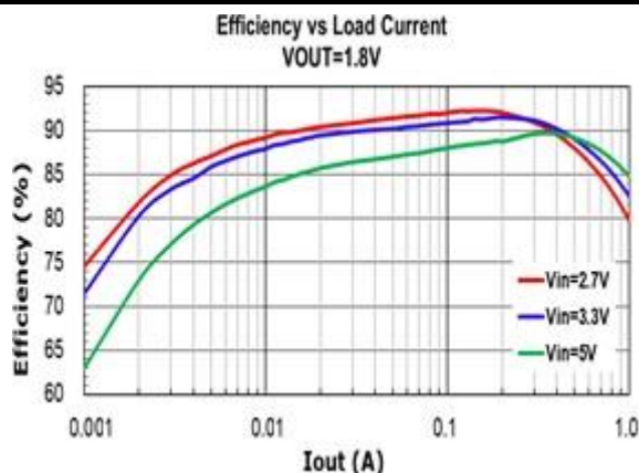
FIG.21 EFFICIENCY V.S. LOAD CURRENT
