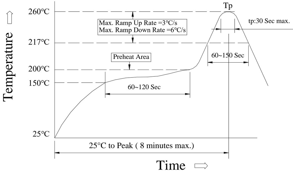
(1) Reflow Soldering Method :
