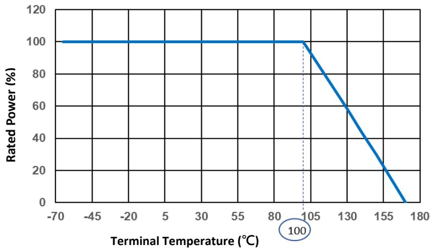
Figure 1. : Power derating curve at terminal temperature
