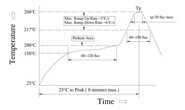
(1) Reflow Soldering Method:
