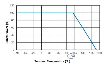
Figure 1. : Power derating curve at terminal temperature
