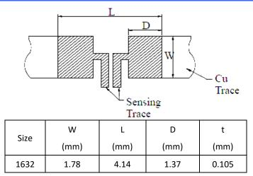
t: Copper toil minimum thickness of PCB
